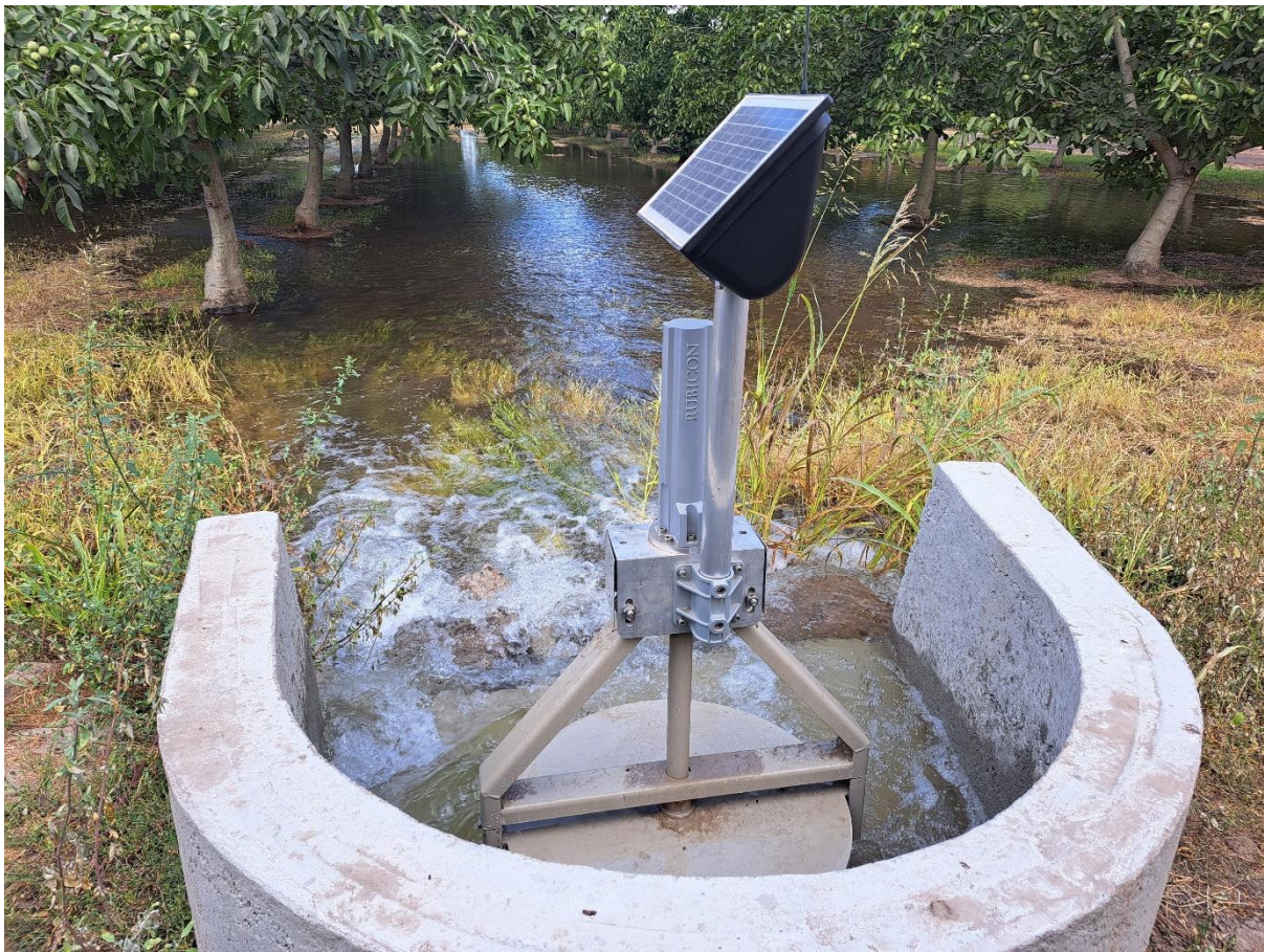
Figure 6 RiserDrive valve automation for alfalfa pipe and riser systems
